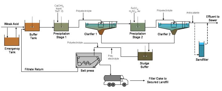
The solid reaction products are dewatered and disposed as compact products in an adequate landfill.
